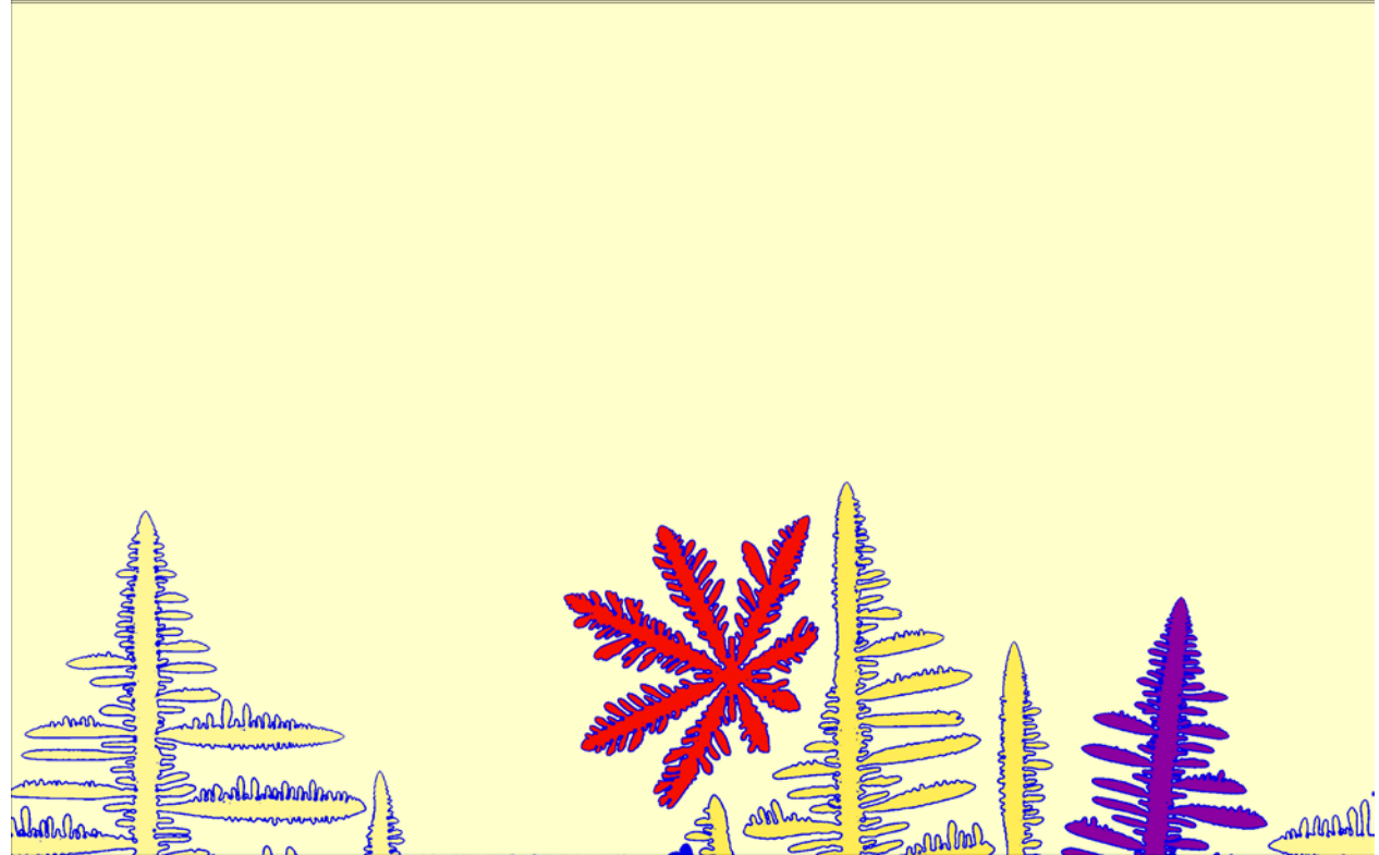
Phase field simulation of CET for the sounding rocket experiment „MACE A“ ( G=7.5K/cm , r=0.2K/s )
