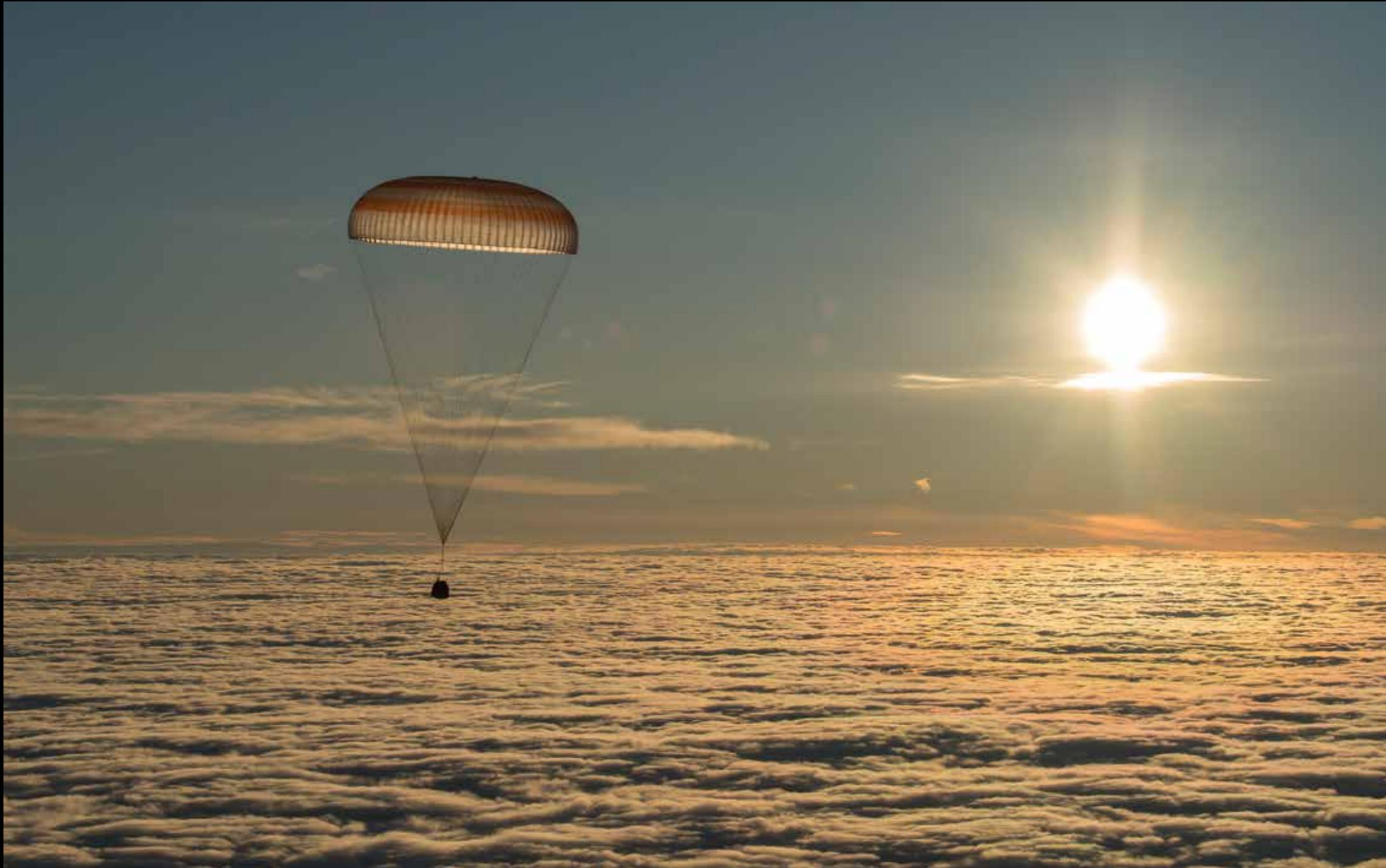
Three hours after leaving the Station, the Soyuz descent module deploys a series of parachutes to allow a stable descent at a speed of around 7 m/s (NASA)
